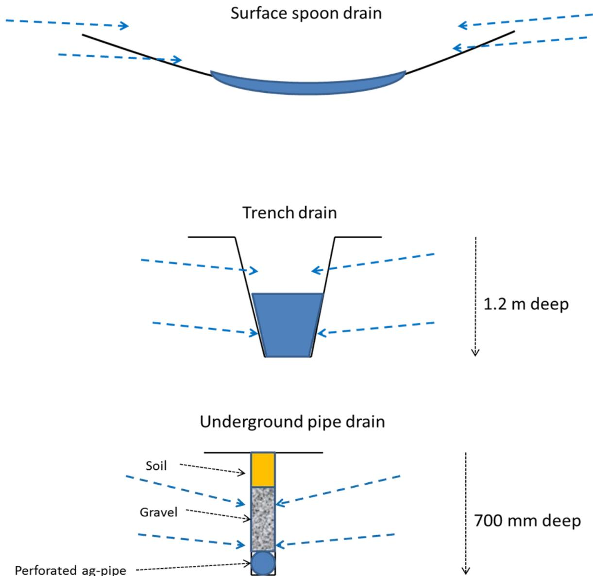
**Figure 3. Characteristics of shallow spoon drain , trench drain and underground pipe drain.**
